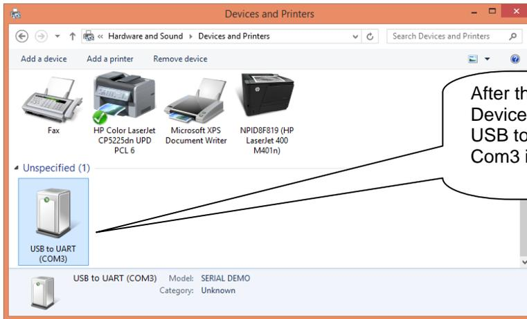
After the driver is updated successfully, the Devices and Printers page will show the USB to UART icon for the 300 USB. It is on Com3 in this example.
