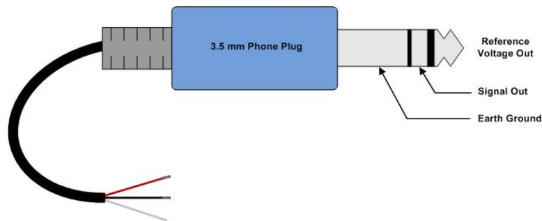
Figure 3. Analog Output Connections
